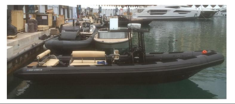
EO WORKBOATS RHIB 8.50 Inboard diesel –waterjet—Yacht version with unique hydraulic bow door.
